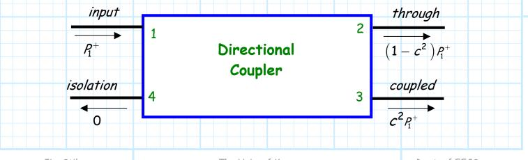
Note however, that **any** of the coupler ports can be an input, with a different through, coupled and isolation port for each case.
