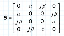
This ideal coupler is **completely** characterized by the **coupling coefficient** *c*, where we find:
